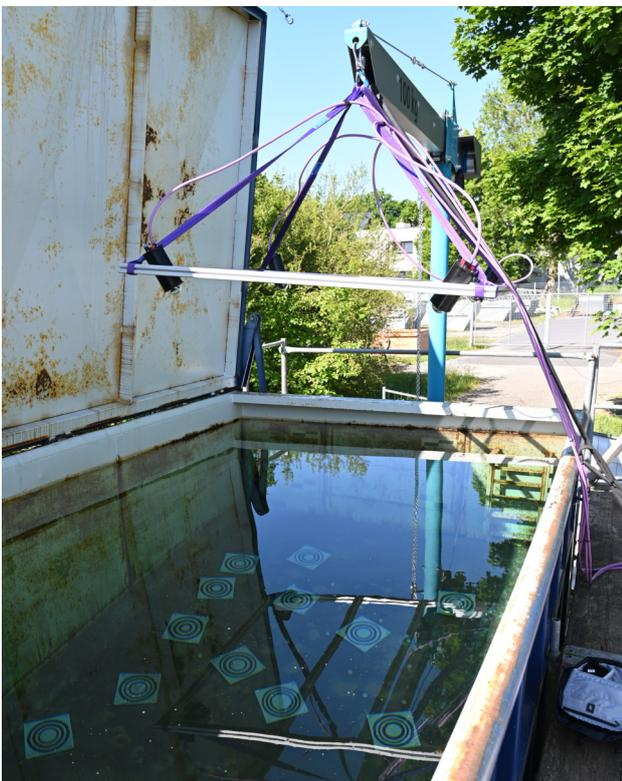
Figure 3. Outdoor setup. Cameras mounted in a square are hung on a crane, looking down towards the water tank.
