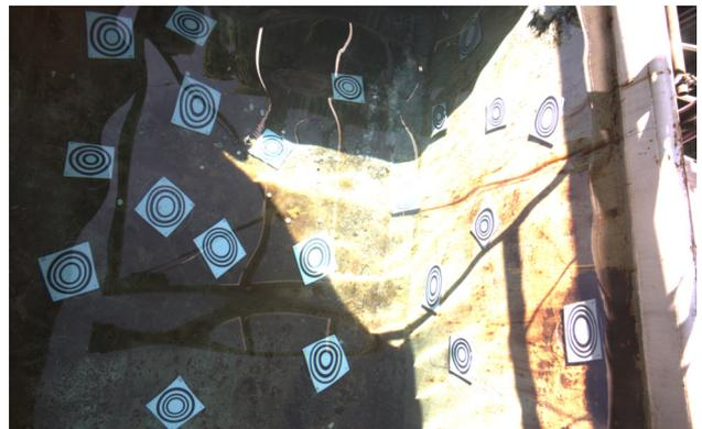
Figure 5. View of one camera with surface distorted by waves, with some fiducials having a distorted appearance.
